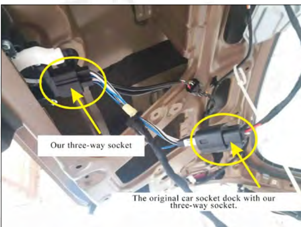
19. Unplug the original car socket and insert our three-way socket (As shown in the figure).
