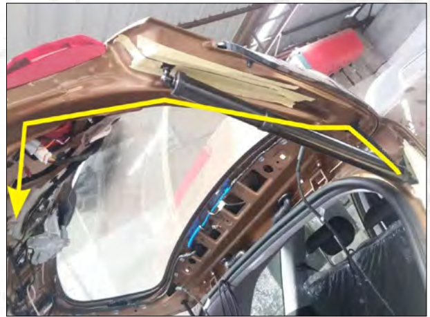
4. Hall line is routed to tailgate (Left and right steps are the same).
