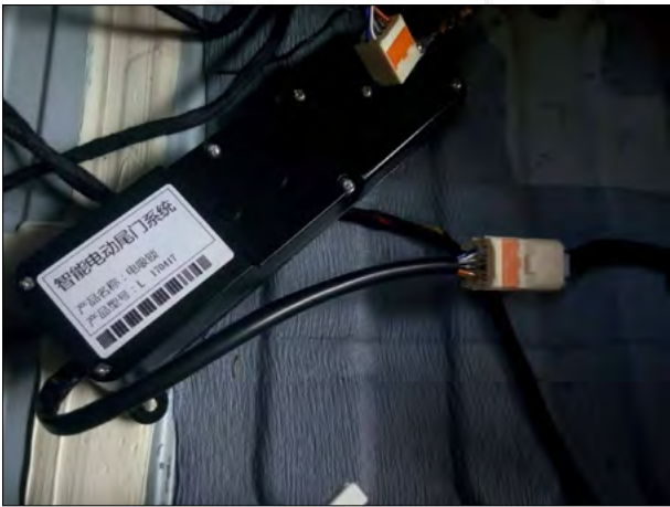
15. Connect the socket of our electric suction cable with the motor socket.
