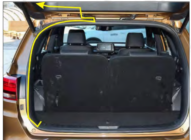
18. The electric suction cable is routed along the yellow line to the central control box of the tailgate cover.
