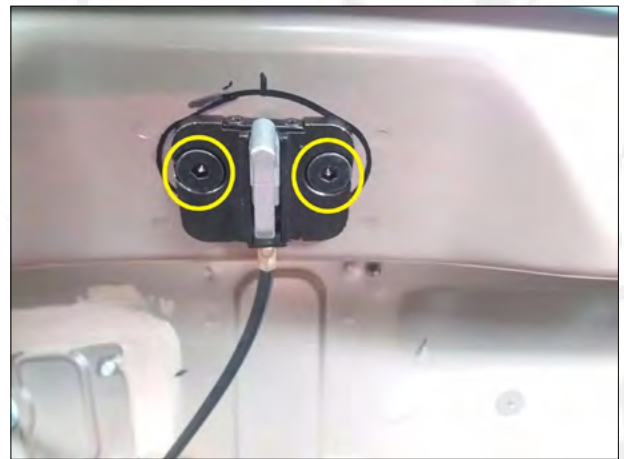
12. Remove the original car lock. Install our electric suction lock and fix it with our screws.
