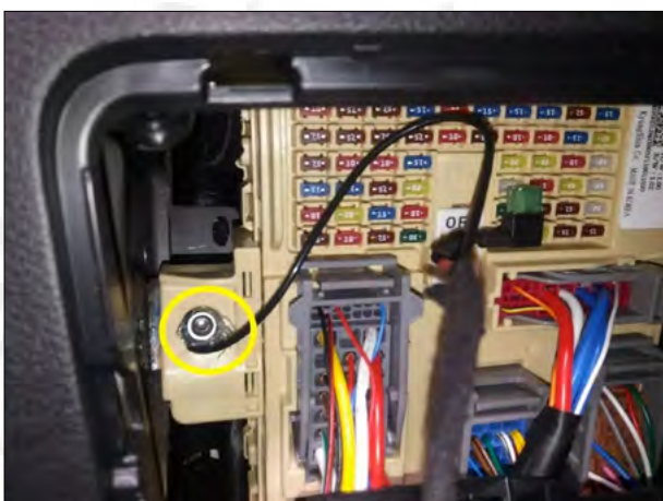
7. Find the ground wire on the left side of the power supply (Shown in figure), connect the ground wire.
