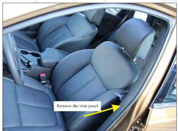
8. Remove the trim panel at the main driver's seat belt B-pillar and find the central control cable.
