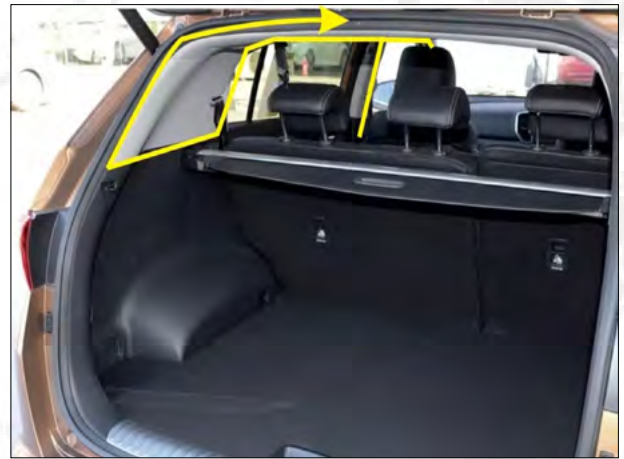
10. Power cable and central control cable follow the direction of the yellow line arrow.
