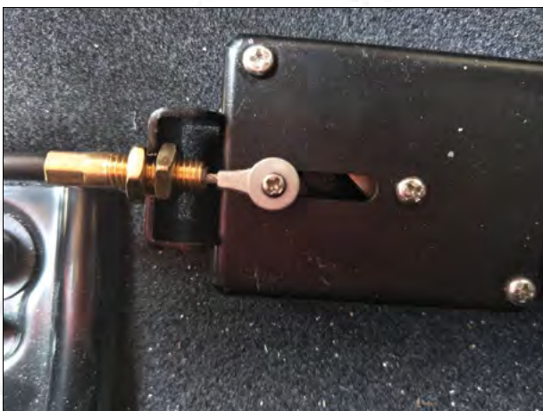
13. Clip the lock rope on the motor. Tighten the screws on both sides and fix it with our screws and gaskets
