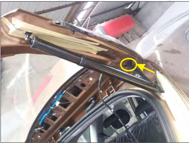
3. Brace Hall line passes through this reserved hole (Left and right steps are the same).
